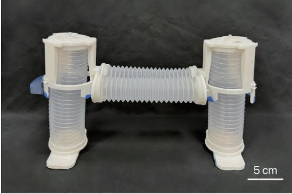
Fig. 1: Adaptive soft pneumatic robot inspired by snake locomotion in this work.
