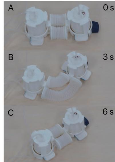
Fig. 9: The robot turning on a wooden board.
