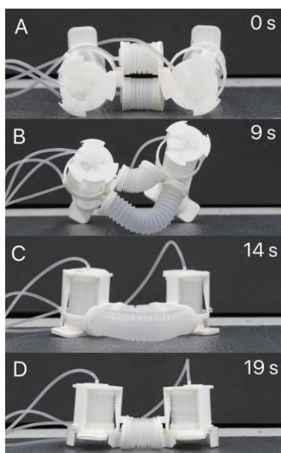
Fig. 11: The robot's self-righting after tipping over.
