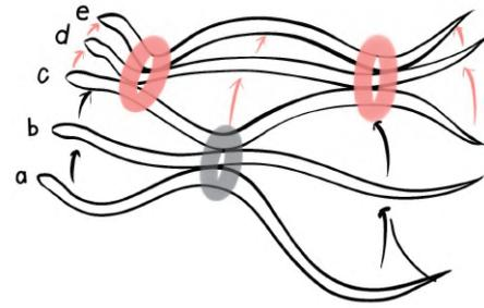
(a) Schematic diagram of the snake's sidewinding locomotion strategy.
