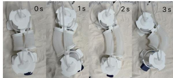
(b) Gait cycle illustration of the robot mimicking the sidewinding locomotion.
