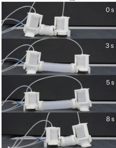
(b) Illustration of the forward locomotion gait cycle of the robot inspired by concertina locomotion.
