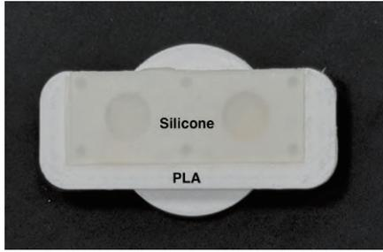
Fig. 3: Bottom view of the silicone footpad.
