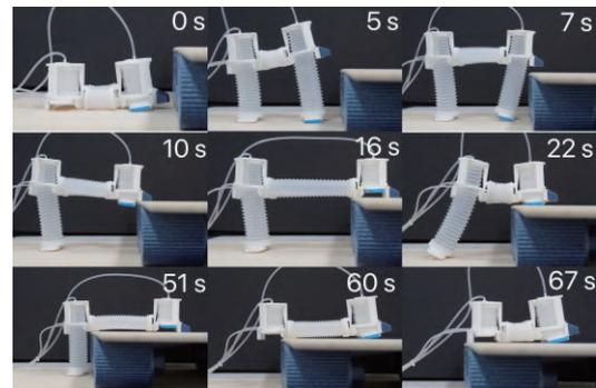
Fig. 7: The process of climbing obstacle.
