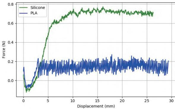
Fig. 4: Friction coefficient tests for silicone and PLA materials of the footpad on a wooden board.
