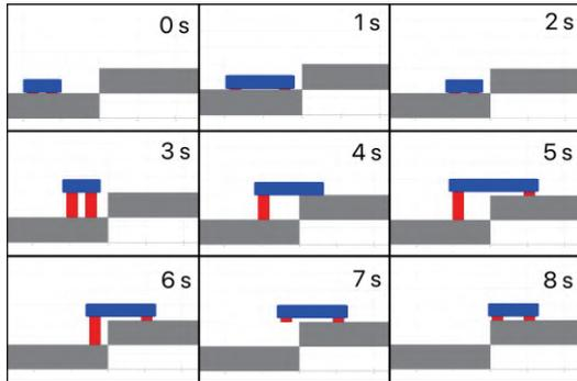
Fig. 8: Matlab simulation of elevation gait.
