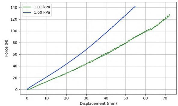
Fig. 2: Experimental results of the soft actuator driven by different pressures under compression tests.
